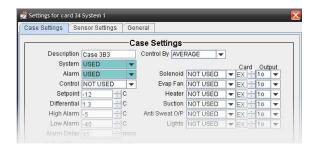
Above: To SHUT OFF Valve (0%) Set the Control to "NOT USED"
