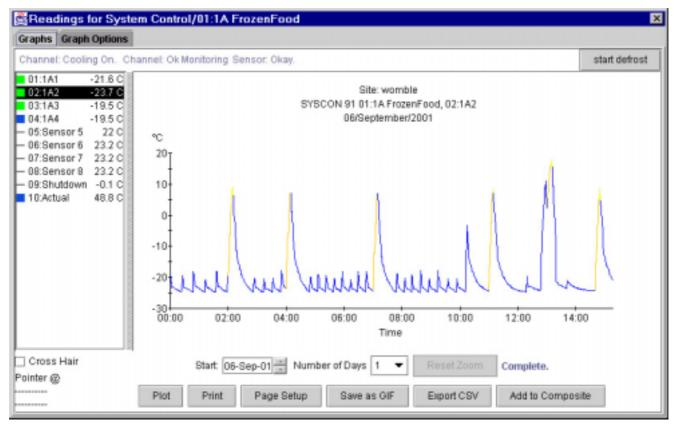
In addition to these excellent specifications, Pressnet adds some very special features- color coded traces allow you to track the system STATUS as well as the parameters (normal condition is a blue trace, alarms are red and defrosts in shades of yellow), so diagnostics of system performance are
