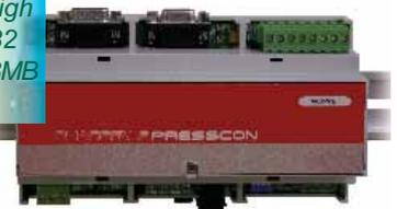
*Power supply 12V DC 5A, includes power filtering & surge protection*
