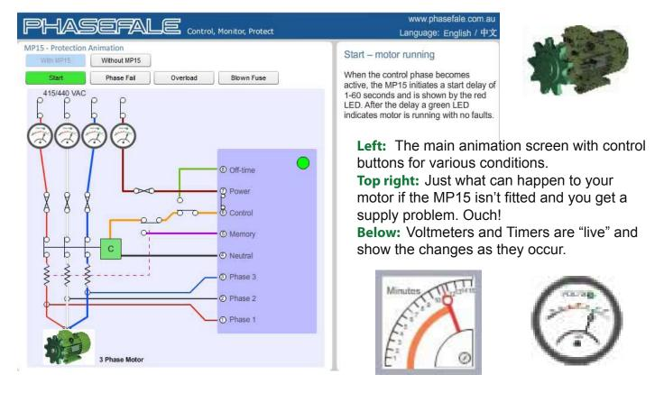
The MP15 Relay animation is a new and exciting way to show you and your customers how the MP15 can protect your motor from all kinds of supply problems. There are separate "buttons" to press which turn on and off the MP15, plus simulate supply problems and the sequence of how the MP15 protects the motor.
