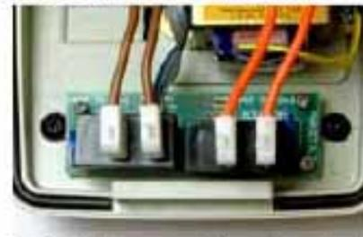
**6** After all electrical connections have been made, with the ELV cables along the top of the main PCB and LV connections across the bottom, the enclosure cover can be fitted in the following sequence:
