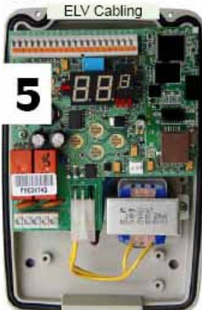
Feed ELV cabling over top edge of board into push fit connectors. Maximum cable size is 0.5mm<sup>2</sup> and strip 6mm bare cable. After fitment, gently tension cable and it is then secure. Route LV cables under bottom left edge and into screw terminals there.
