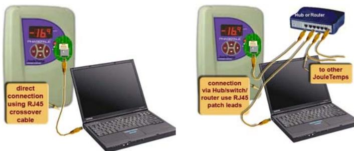
Above: connecting your JouleAlarm to a laptop or PC via direct connection or via a switch/hub/router
