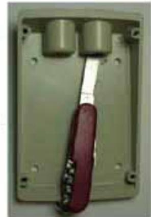
For maximum safety, bring LV mains cables (e.g. 240 V AC supply, compressor/evaporator control, fan, heater and alarm light) in through a different conduit than the Extra Low voltage cables (e.g. Sensor cable, alarm isolate, defrost terminate, alarm buzzer and security etc.)
