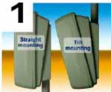
**1** Decide if you want straight (left picture) or tilt mounting. The wall mount conduit entry points are at the bottom for straight mount and at the top for tilt (approx 15 degrees) mounting.
